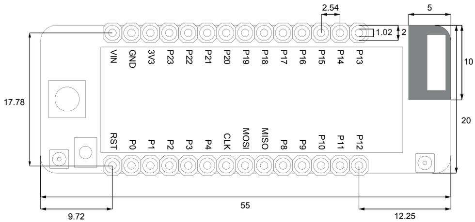
Figure 4 – Mechanical drawing (top down view) – Units: mm
