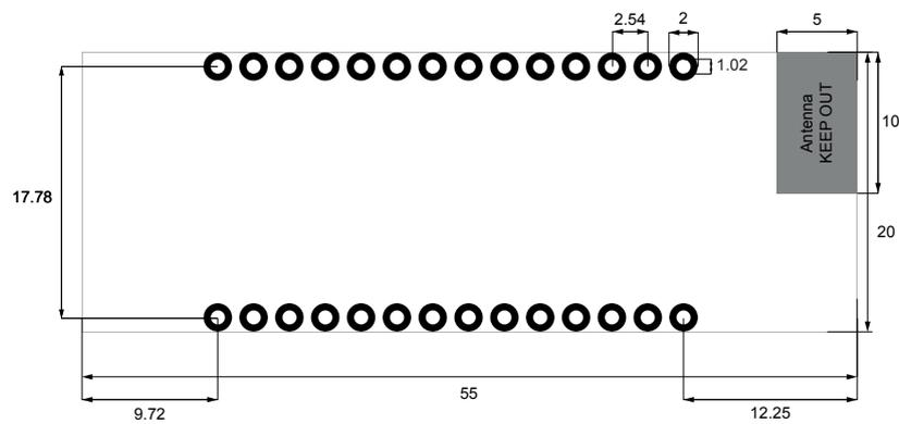
Figure 6 – Recommended land pattern (through hole) – Units: mm
