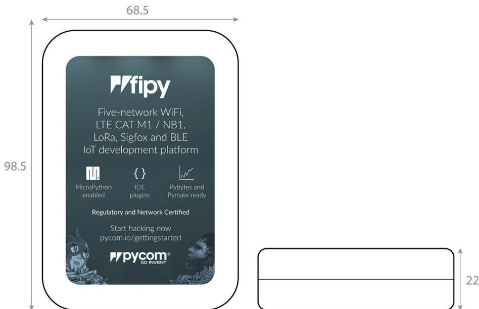
Figure 7 – Mechanical drawing of packaging – Units: mm
